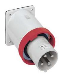
Flush-mounting plug, PLUSO series, 3 poles + PE, 6 h (red), 63 A, 380  $\div$  415 V
