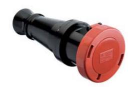
Mobile socket outlet, PLUSO HEAVY DUTY series, 3 poles + N + PE, 6 h (red), 63 A, 380 ÷ 415 V
