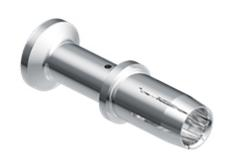
Female crimp contact, CX7 series, 70 A, turned silver plated, wire cross section 10  $\text{mm}^2$ , AWG 8 - 7
