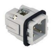
Male insert, JK series, screw terminal connection, 3 poles + PE, 10 A 230/400 V 4 kV 3, size "21.21"
