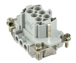
Female insert, JNE series, screw terminal connection, 6 poles + PE, 16 A 500 V 6 kV 3, size "44.27", with plate
