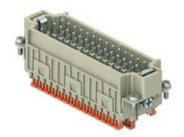
Male insert, CDSH series, SQUICH® spring terminal connection without tools, 42 poles + PE (43-84), 10 A 400 V 6 kV 3, size "104.62"
