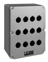
Box for control devices and signals, AC series, M32 cable entry, 12 holes for unit Ø 22 mm, external dimensions 152x205x102 mm
