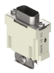
Male modular insert. Mixo Data series. D-SUB. 9 poles, 1 module, 5 A 50 V 0,8 kV 3, crimp, shielded, 2 cable entries
