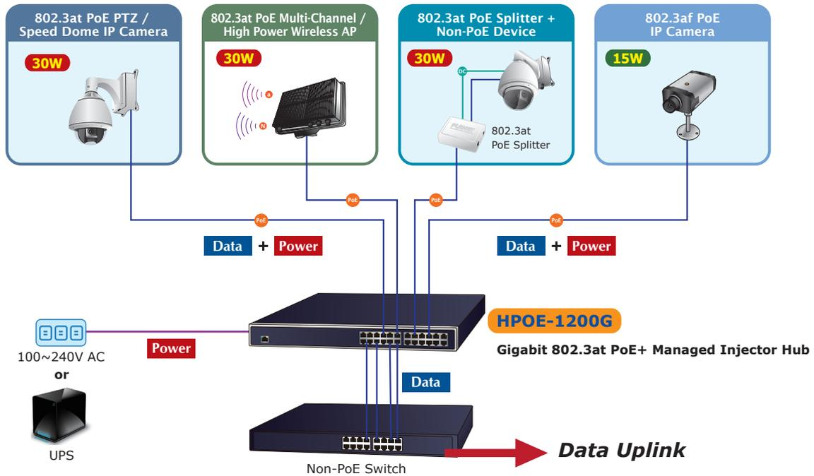
With data and Power over Ethernet from one unit, the HPOE-1200G can reduce power cable deployment and eliminate the need for dedicated electrical outlets on the wall, ceiling or any unreachable place.
