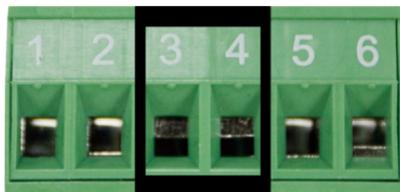
Figure 7: Fault Pin of Terminal Block.
