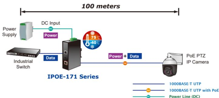
**Figure 9:** Architecture of connected IEEE 802.3at/bt device
