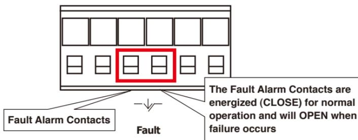
Figure 8: Fault Alarm Contact
