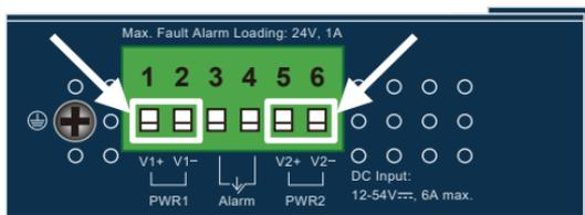
Figure 5: Power input pins.
