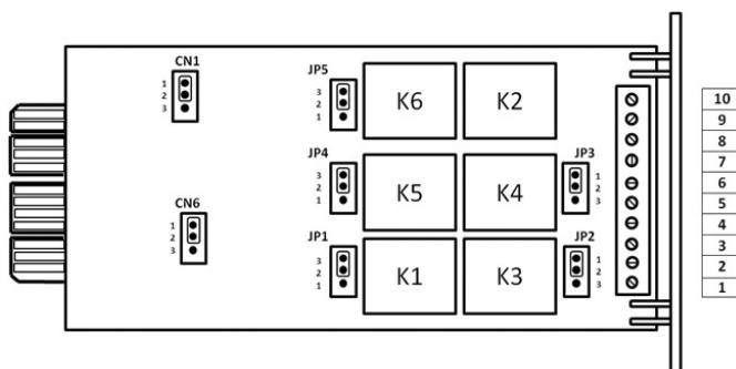
The card is made up of 6 relays (K), of 5 configuration jumpers (JP) to select the normally open or normally closed dry contact and 2 configuration jumpers (CN) to select the mode of the remote UPS shutdown.
