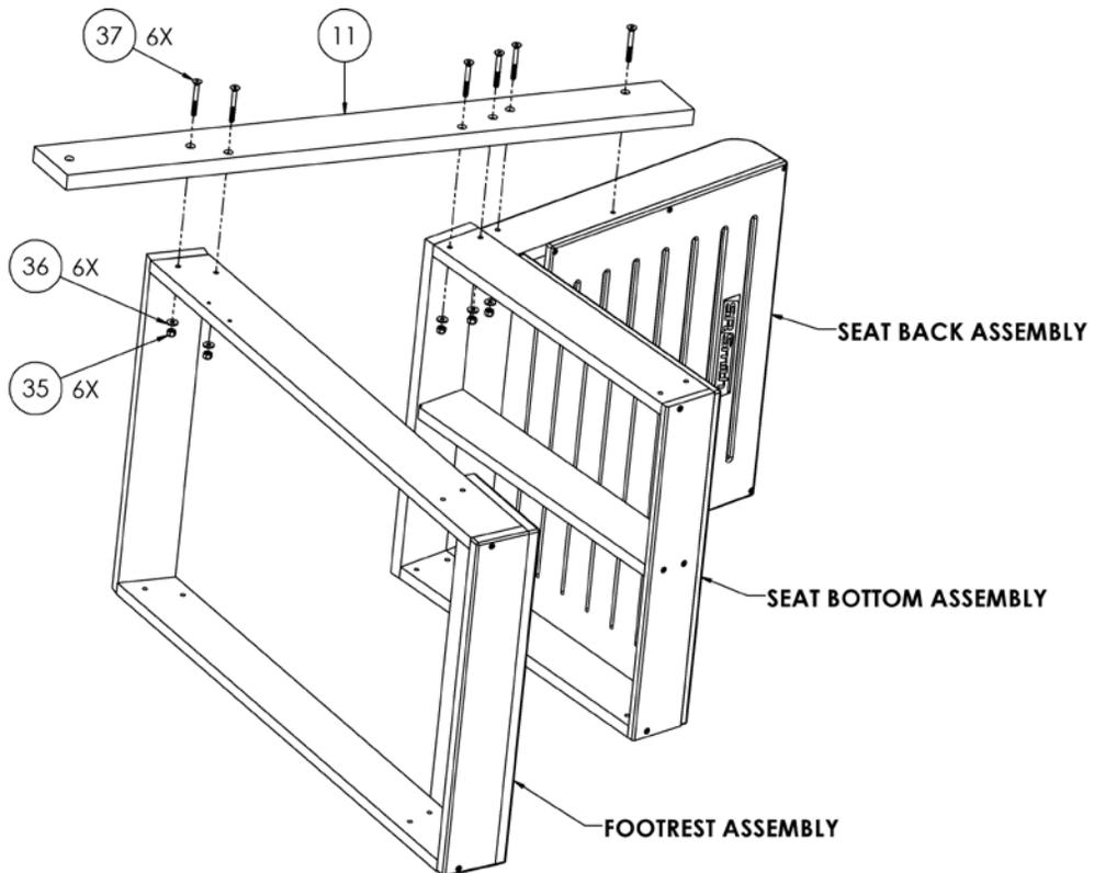
16. Next, attach leg (9) to assembly using nuts (35), washers (36), and screws (37).
