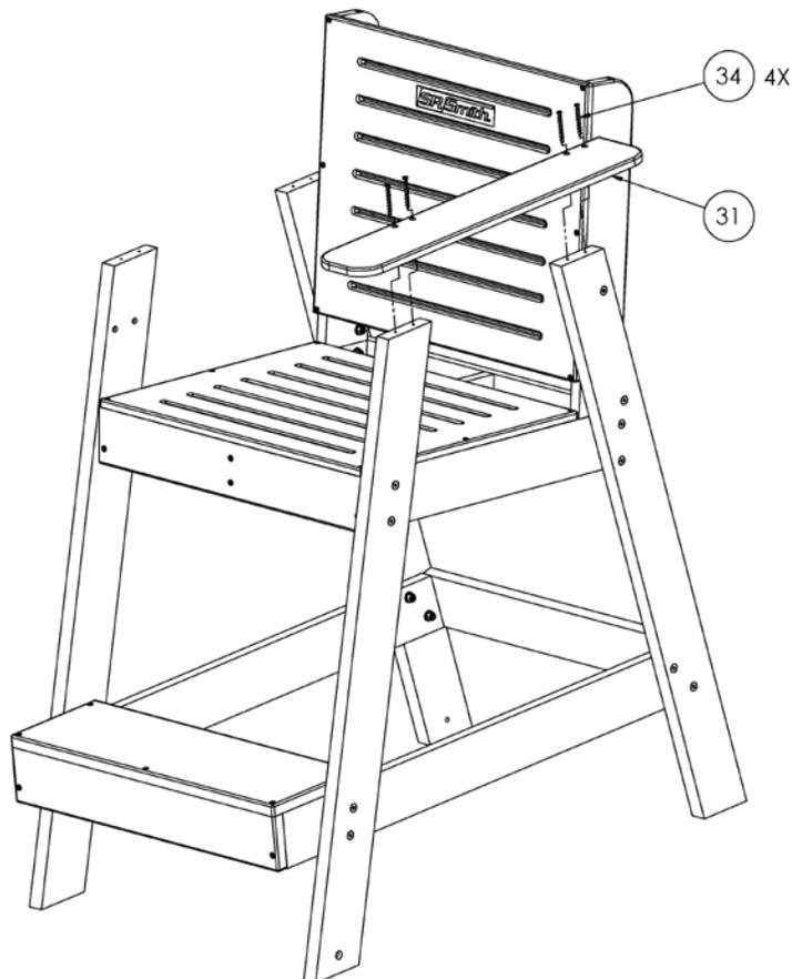
20. Attach right arm (32) to assembly with screws (34).
