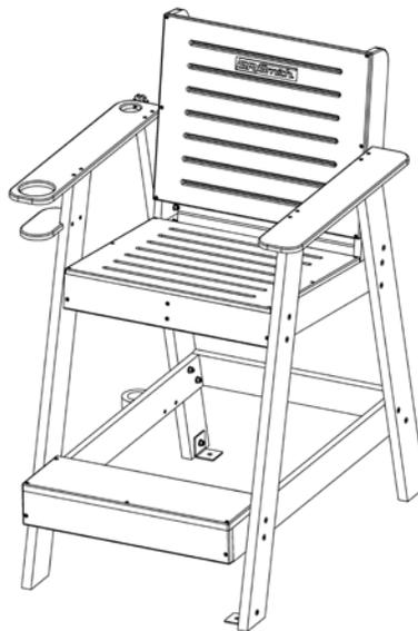
**Warning:** Chair required to be anchored to deck when using umbrella.
