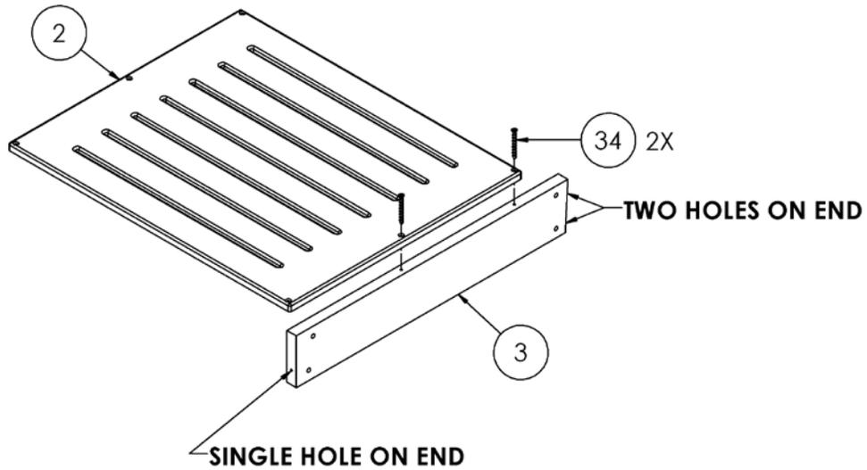
2. Attach part (3) to assembly using screws (34).
