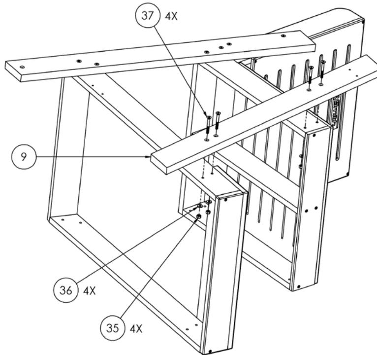
17. Flip chair and attach leg (12) to assembly using nuts (35), washers (36), and screws (37).
