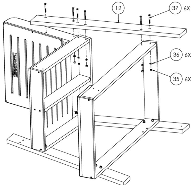
18. Next attach leg (10) to assembly using nuts (35), washers (36), and screws (37).
