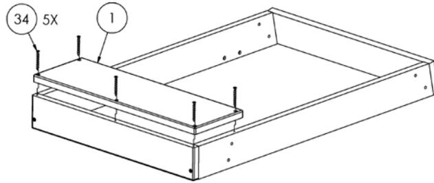
14. Finished Footrest Assembly should look like the picture below. Next attach legs using last 3 assemblies.
