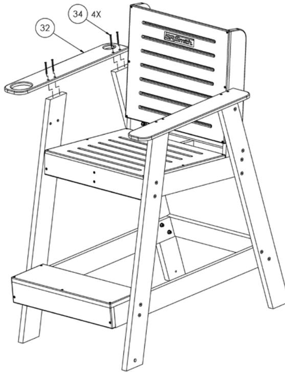
21. Install cup holder (27) using screws (34).
