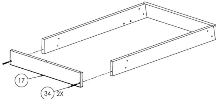
13. Attach part (1) to assembly using screws (34).
