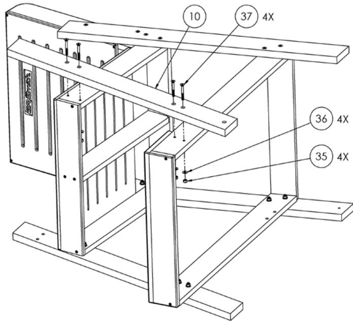
19. Now attach left arm (31) to assembly using screws (34).
