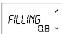
During the filling stage, the **ORIMUM PILOT** indicates the pressure measured in the heating circuit.
