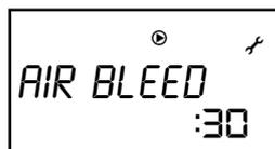
The purging cycle activates the circulator pump (and the 3-way valve if production of domestic hot water is also installed) at an alternating rhythm to allow the displacement and purging of any air bubbles accumulated at high points of the installation using the **ORIMUM PILOT's** automatic purger.
