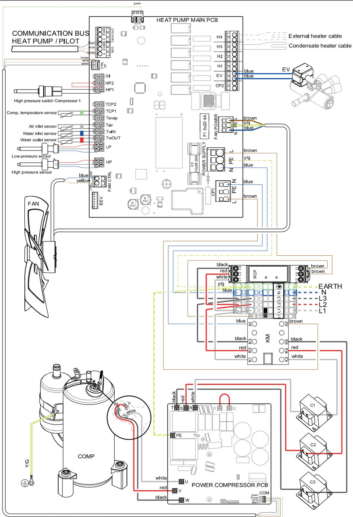
*TwOUT* - Water outlet temperature sensor
