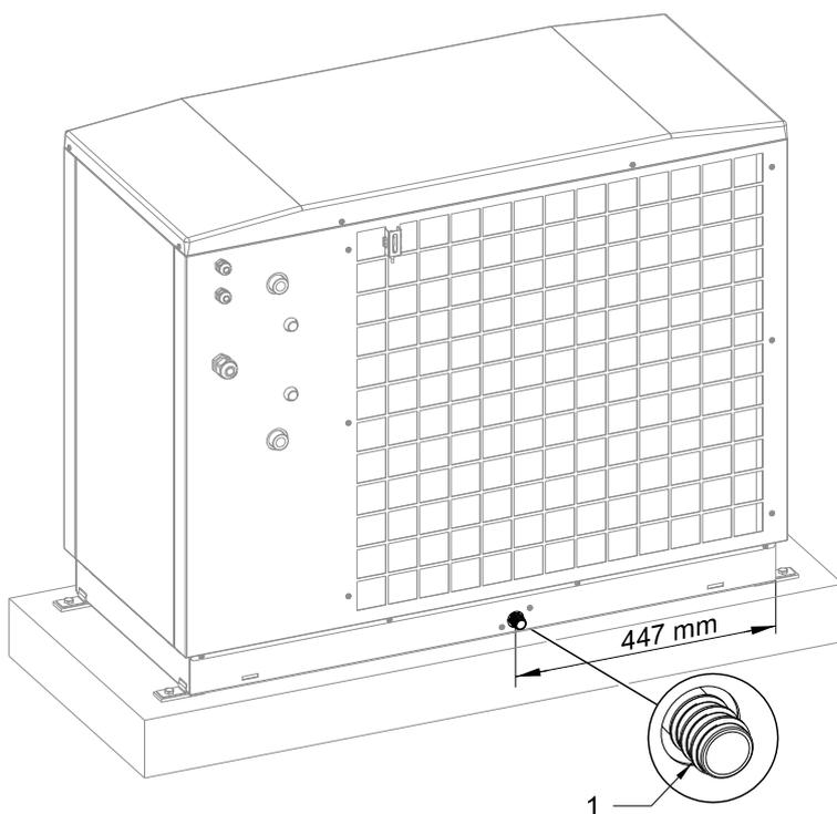
When the appliance is operating in frost protection mode, the condensed water must be drained off. In order for the condensates to drain properly, the drainage trough and hole 1 must be clean and free of all debris (leaves, grass, etc...).
