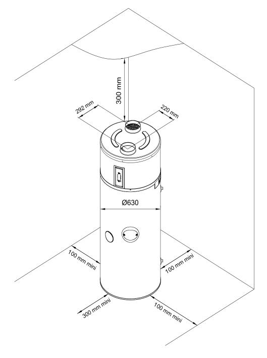
• The floor must be able to support the weight of the domestic hot water heat pump (weight of the domestic hot water heat pump filled with water 250 L= 335 kg).
