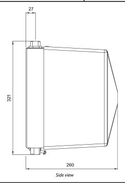
2.3.1 - Dimensions with one circuit 2 (mixed) (standard model)
