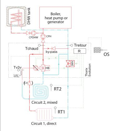
MANDATORY in cases where circuit n°2 is an underfloor heating circuit.
