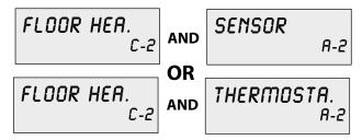
3.4.7 - Power supply to boiler controlled by 65°C safety aquastat where the secondary circuit is an underfloor heating circuit
