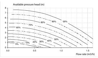
Power absorbed 4 to 70W depending on the speed. Input current 0.05 to 0.58A depending on the speed.
