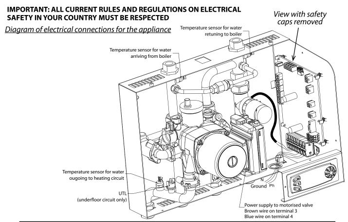
The terminal strips are spring-loaded «Cage Clamps». For handling, use a 3.5 x 0.5mm screwdriver.
