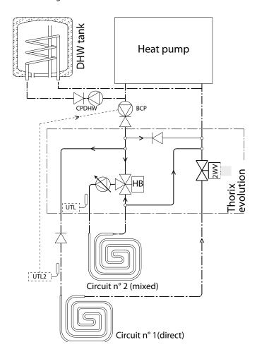
ВН Hydraulic block with low-energy, variable-speed circulator pump and a motorised 3-way valve
