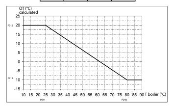
The target temperature for the leaving water from the 3-way valve is deduced from the temperature read by the "T boiler" sensor:
