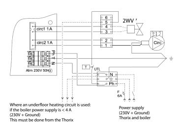
3.4.7.2 - Boiler with  $\geq$  4A power supply or high temperature heat pump (>65°C) or heat pump with boiler or electrical back-up
