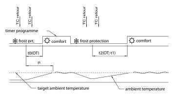
The initial heating advance = t0 = 4 hours in the underfloor heating circuit and 45 minutes in modulated radiators, depending on the outdoor temperature (OT). Successive heating advance periods are calculated using the following formula:
