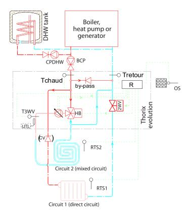
MANDATORY in cases where circuit n°2 is an underfloor heating circuit.
