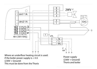
3.4.7.2 - Boiler with ≥ 4A power supply or high temperature heat pump (≥65°C) or heat pump with boiler or electrical back-up
