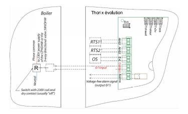
This connection is optional in cases where the generator is equipped with a 3-way valve which ensures a total switch to domestic hot water production when requested.
