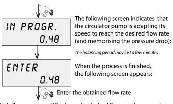
(this flow rate may differ from the desired flow rate because the circulator pump speed variation is not continuous, but adjusts gradually in stages of 10%).
