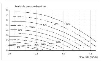
Power absorbed: 4 to 70W depending on the speed. Input current 0.05 to 0.58A depending on the speed.
