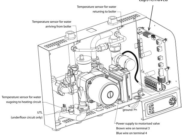
The terminal strips are spring-loaded «Cage Clamps». For handling, use a 3.5 x 0.5mm screwdriver.
