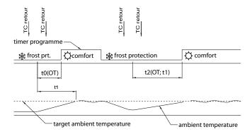
The initial heating advance = t0 = 4 hours in the underfloor heating circuit and 45 minutes in modulated radiators, depending on the outdoor temperature (OT).
