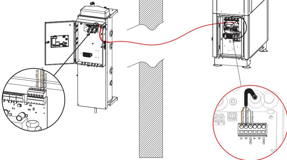
Plan for the appropriate length of cable between the pilot and the heat pump. Do not hesitate to cut the cable to the appropriate length to **AVOID LOOPS**.
