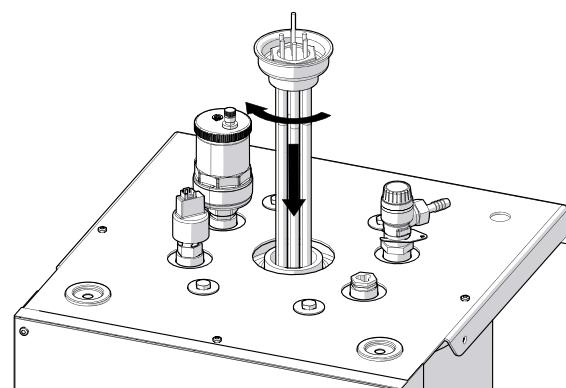
3. Insert and screw on the electrical back-up heater using a 60 mm open-end wrench, ensuring a watertight seal during connection.
