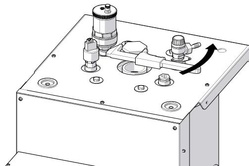
2. Remove the plug above the tank using a 49 mm open-end wrench.
