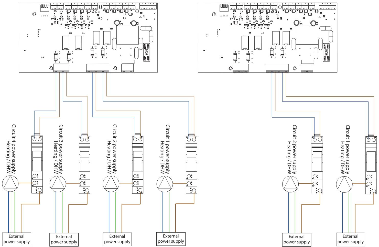
In this case, the circulator must have its own power supply. Do not supply the circulators from the **Z1 Pilot**.
