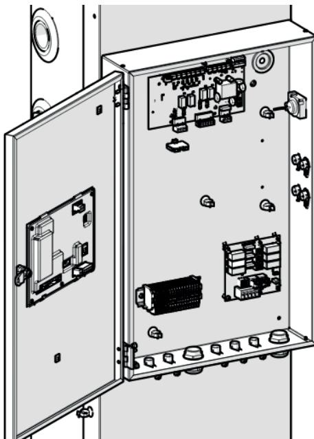
6. Connect the three electrical resistor power connectors to the power board. Check the electrical continuity of the electrical back-up heater terminals with a multimeter to identify each resistance. Screw the phase and neutral of each connector to the terminals with electrical continuity using a torque wrench. Tightening torque should be 1.1 N.m.
