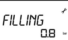
During the filling stage, the **Pilot** indicates the pressure measured in the heating circuit.
