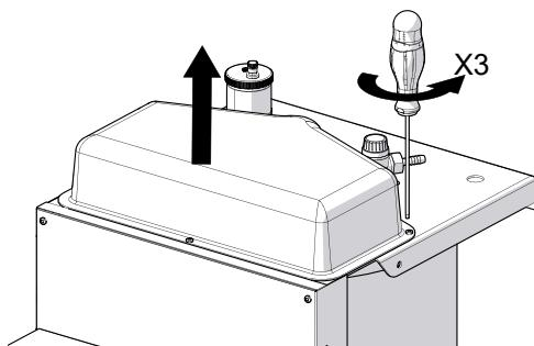
1. Remove the cover above the pilot using a Torx T20 screwdriver.
