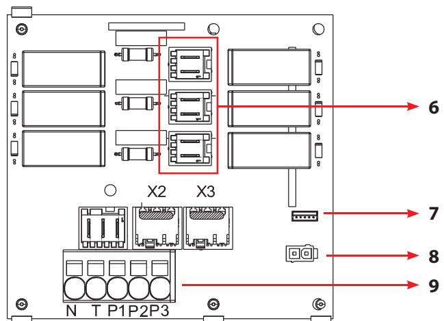
For single-phase connection, the phase must be connected to terminal **P3**.
