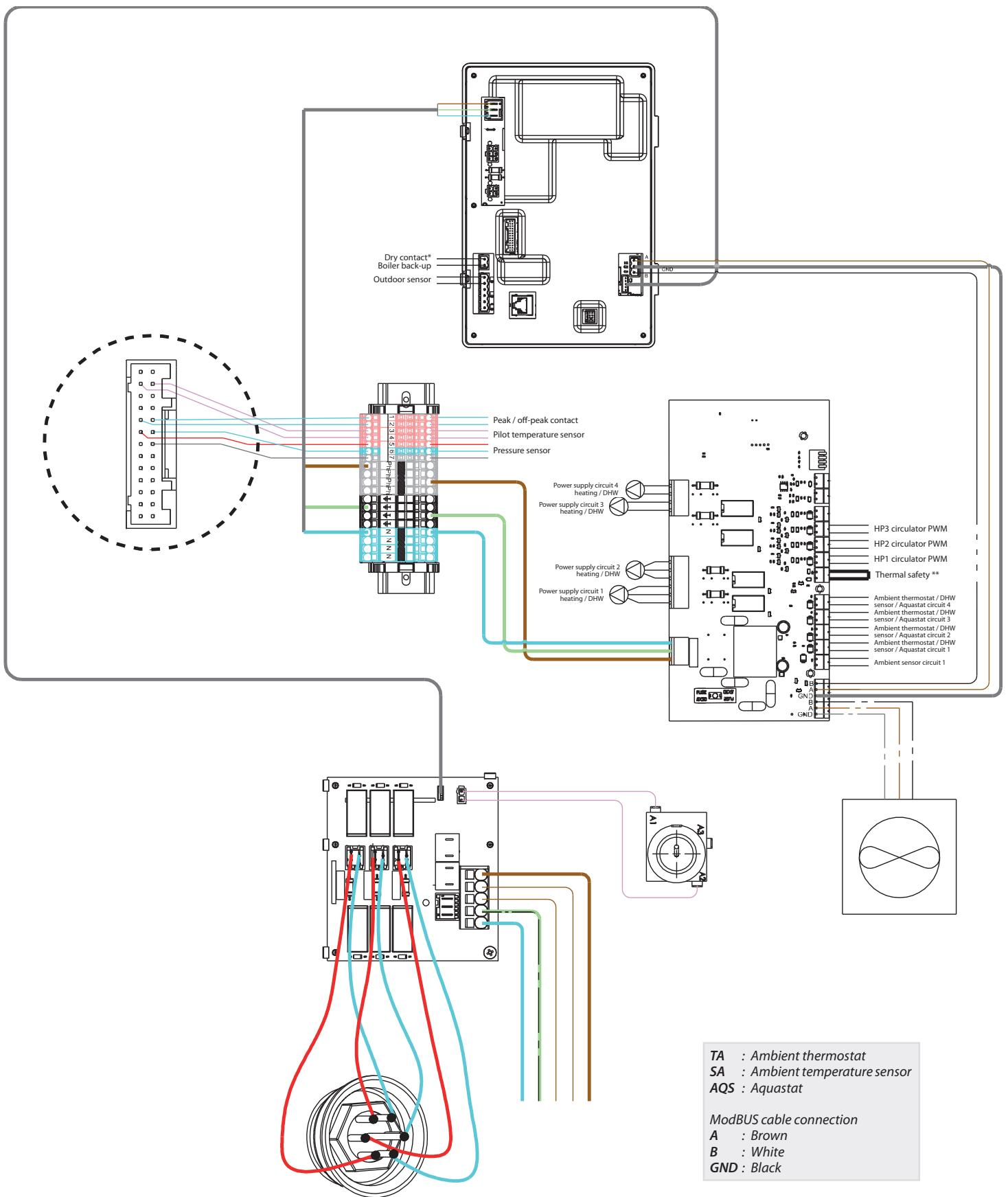
\* Dry contact to be connected to room control input of boiler back-up.
