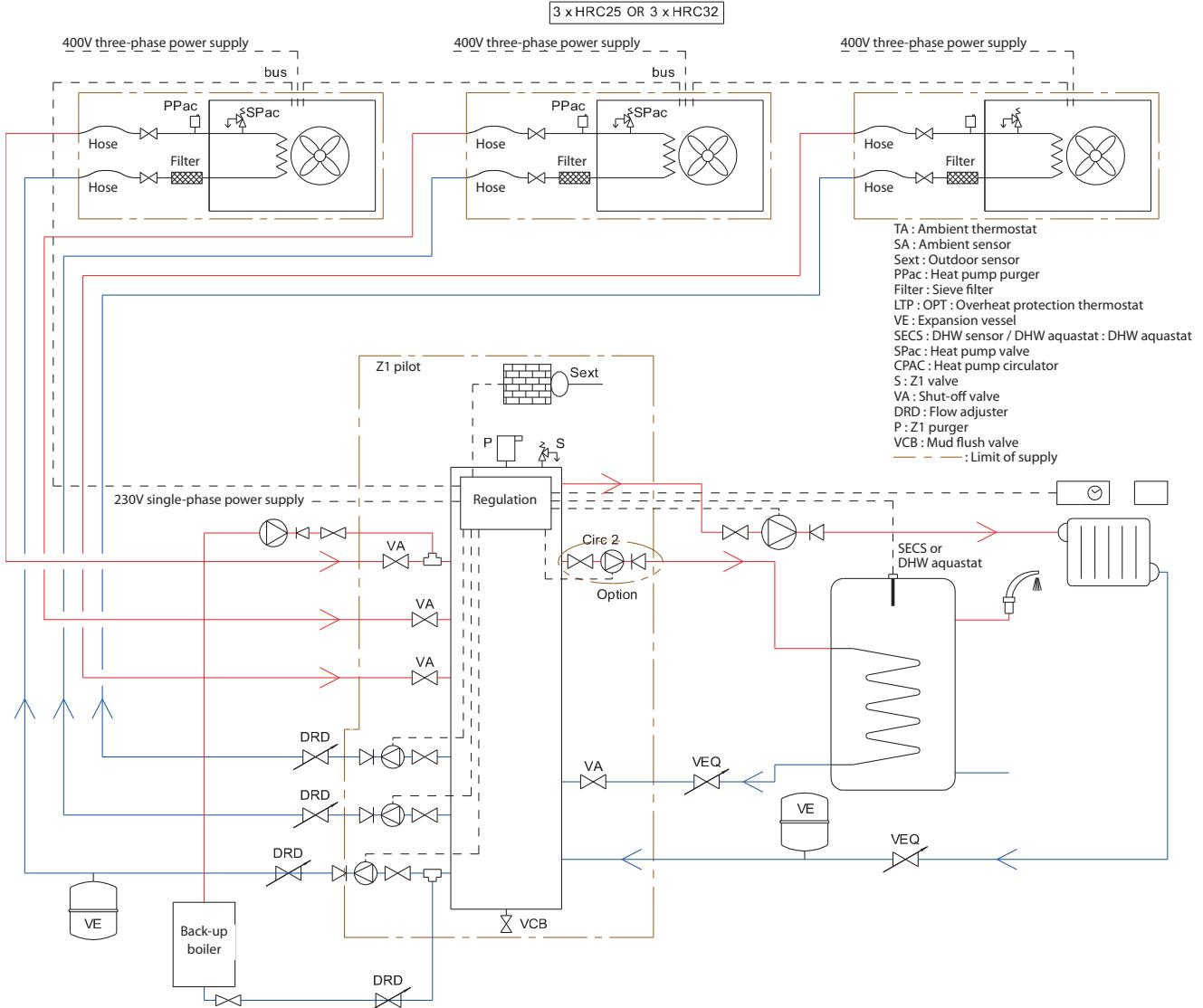
If the circulator installed on the emitter circuit(s) is not the one supplied in the AUTO hydraulic branch (Ref. 755823), install a relay between the control board and the circulator as follows:
