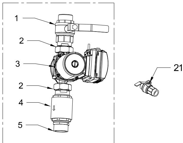
**B: AUTO hydraulic branch for transmitter circuit(s)
