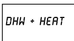
simultaneous programming of heating and domestic hot water
