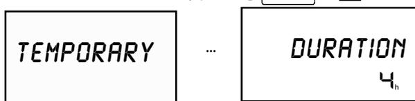
Temporary comfort mode can be programmed to last from 1 to 72 hours.
