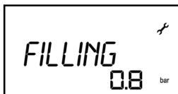
During the filling stage, the **Pilot** indicates the pressure measured in the heating circuit.
