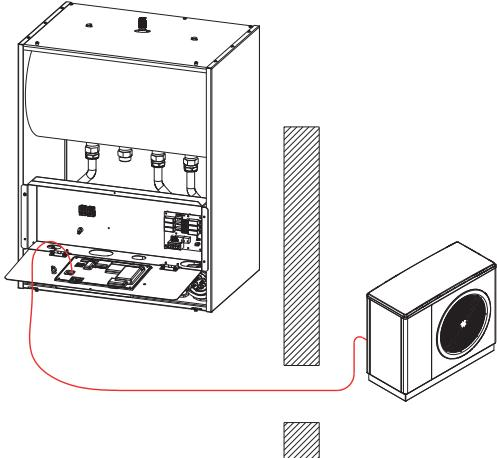
Plan for the appropriate length of cable between the pilot and the heat pump. Do not hesitate to cut the cable to the appropriate length to **AVOID LOOPS**.
