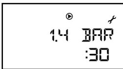
During the purging cycle, the screen indicates the countdown until the automatic stop of the cycle as well as the pressure in the circuit.
