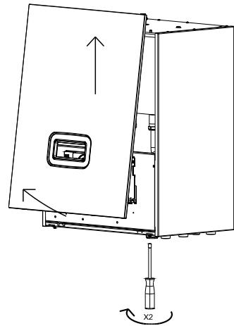
1- To remove the front panel, unscrew the two TH7 screws which are located on both sides underneath the **Pilot**.
