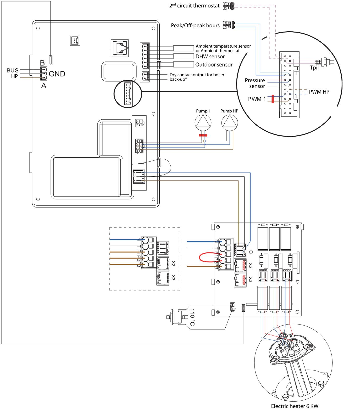
\* Dry contact to be connected to the ambient thermostat input of the boiler back-up.
