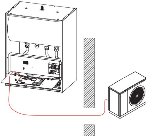
Plan for the appropriate length of cable between the pilot and the heat pump. Do not hesitate to cut the cable to the appropriate length to **AVOID LOOPS**.
