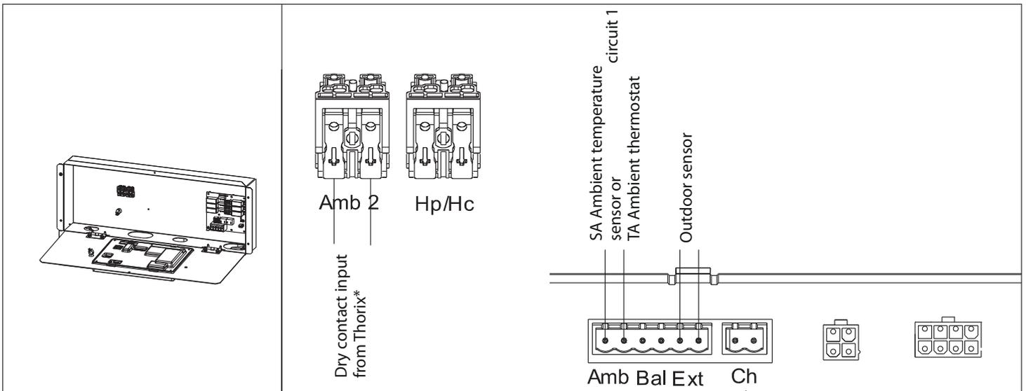
\* On the Thortex module, connect the two wires to the Alarm output and set P219=1.
