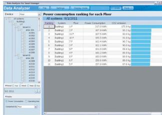
Quickly spot high consumption air conditioners by displaying power consumption ranking.
