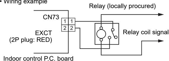
**Note)** Determine the cable length between the indoor, outdoor control P.C. board and the relay so that they are within 2 m.
