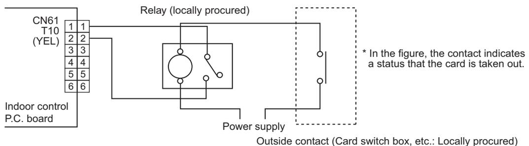
Note) Determine the cable length between the indoor control P.C. board and the relay so that they are within 2 m.
