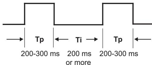
The terminal can input a pulse signal.
