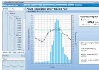
More than just power consumption, simultaneously display outdoor temperature, room side suction temperature, and indoor set temperature which affect power consumption. Plus it is possible to analyze operating status by month, date, and time.
