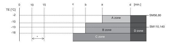
\* From 10 minutes to 15 minutes after a heating operation started, the minimum value of TE is stored in memory as TEO and the minimum temperature of TO as ToO.
