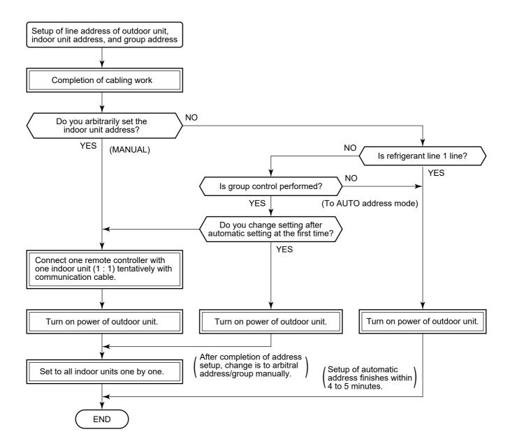
ë When the following addresses are not stored in the neutral memory (IC503) on the indoor P.C. board, a test run operation cannot be performed. (Unfixed data at shipment from factory)
