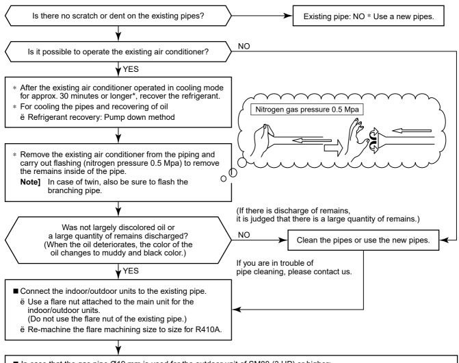
■ In case that the gas pipe Ø19 mm is used for the outdoor unit of SM80 (3 HP) or higher: (Gas pipe size of our R410A model 3 is Ø15.9 mm)
