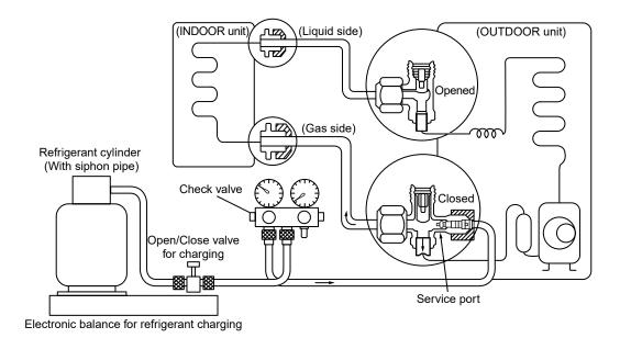
Fig. 6-4-1 Configuration of refrigerant charging
