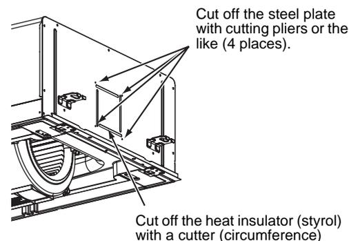
**2** A gap between the styrol and steel plate may cause a trouble such as condensation. Be sure to attach the attached heat insulator A first with it aligned to the screw hole, and then attach seal heat insulator B, according to the following figure.
