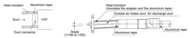
5 Insulate 2 ducts to the outside and the SA (supply air) using a heat insulator to prevent condensation.
