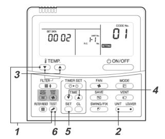
1 Push ∌ button and temp. setup ▼ button simultaneously for at least 4 seconds.
