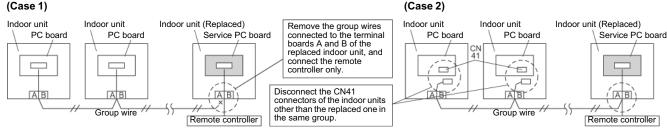
After the \*3 procedure is complete, restore the group wires or CN41 connectors removed temporarily.
