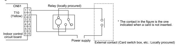
Note: The length of the wire between the indoor control circuit board and relay should be 2 m or less.
