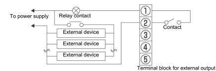
Connect to the terminal block for external output (1 and 2) in the electrical control box Connection wire (locally procured): 2-core wire (H07 RN-F or 60245 IEC 66) 1.0 mm<sup>2</sup> to 2.5 mm<sup>2</sup>
