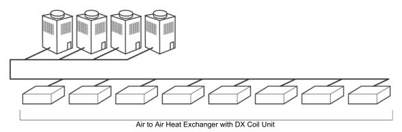
The Air to Air Heat Exchanger with DX Coil Unit and the concealed duct type fresh air intake unit cannot be used together in the same system.
