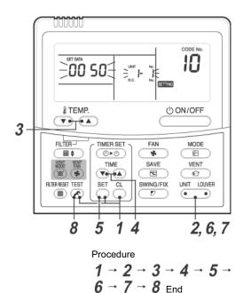
Checking all the indoor unit addresses using a wired remote controller (Available when the address has already been set)
