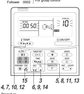
\*1 Do not set the address 29 or 30 if the line address is set using the remote controller.
