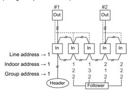
Release the remote controller wiring, connect the wired remote controller and then set the addresses.
