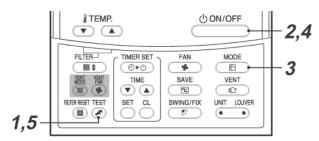
When the TEST button is pressed and held for at least 4 seconds, "TEST" appears on the display, and the test run mode is established.
