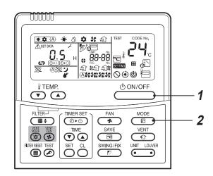
Press the buttons to start operation. The operation lamp lights up.
