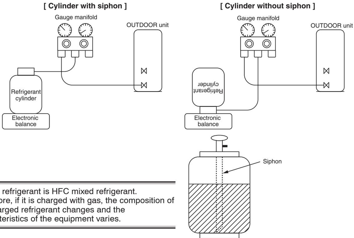
R410A refrigerant is HFC mixed refrigerant. Therefore, if it is charged with gas, the composition of the charged refrigerant changes and the characteristics of the equipment varies.
