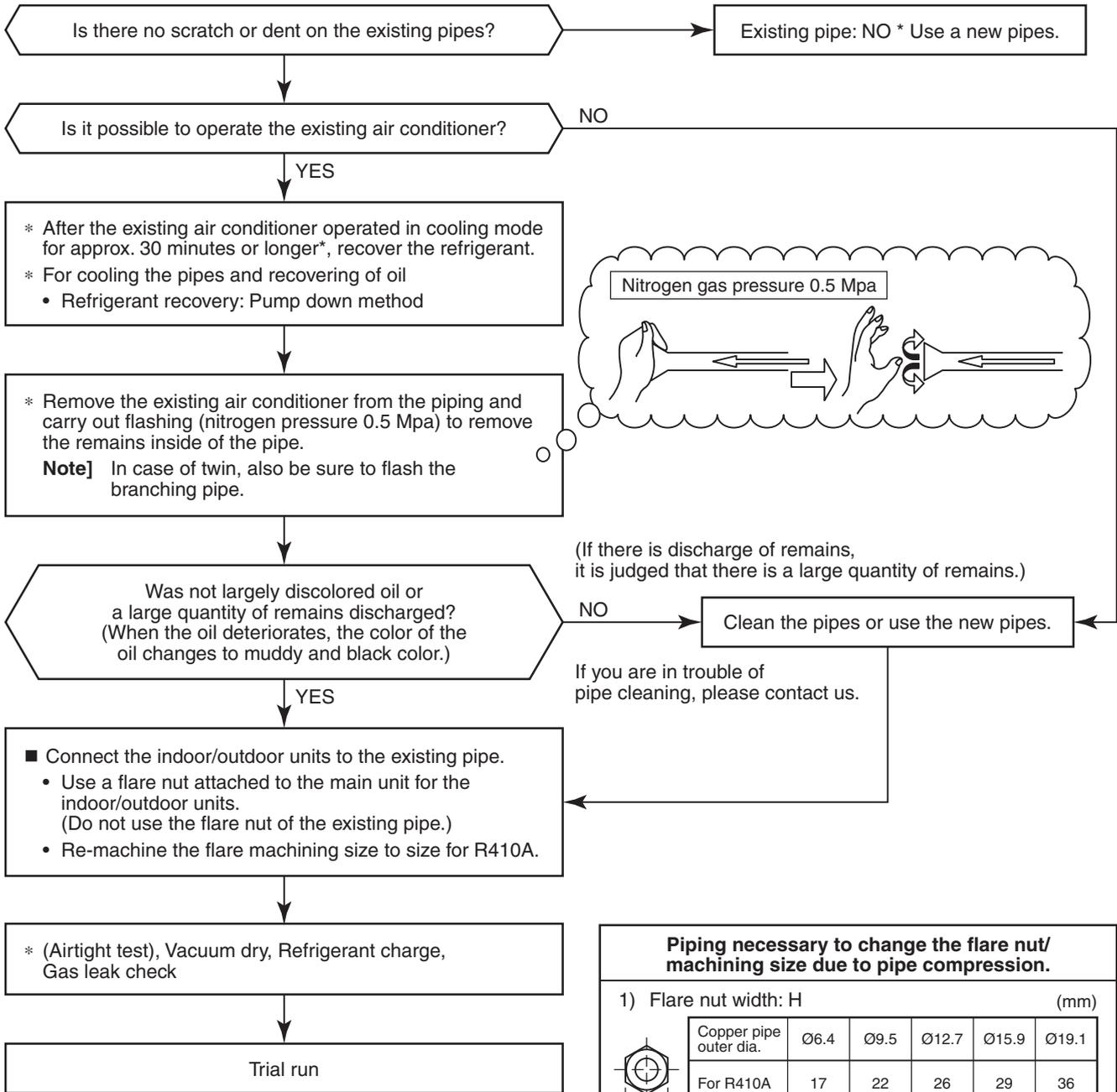
**Piping necessary to change the flare nut/ machining size due to pipe compression.**
