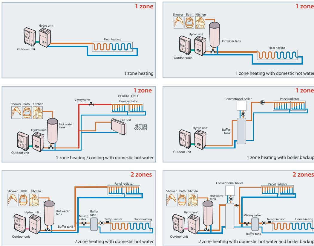
In existing dwellings already equipped with traditional gas or fuel boilers, Toshiba Estia air to water heat pump system can be combined with the existing heating system to cover exclusively and in an optimized way all the heating needs, all year round. Then, the boiler is only used as a back-up source during some extreme weather days of the winter.
