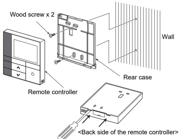
1 Insert a flat-blade screwdriver into the groove on the back side of the remote controller to remove the rear case.
