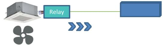
(Note) Signal is OFF when 4-way cassette type performs intermittent operation after oil recovery control.
