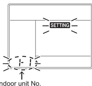
**2 Each time [ ∇ ] [ △ ] setting button is pushed, indoor unit numbers in the group control change cyclically. Select the indoor unit to change settings for.**
