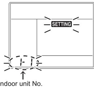
**2 Each time [ ∇ ] [ △ ] setting button is pushed, indoor unit numbers in the group control change cyclically. Select the indoor unit to change settings for.**
