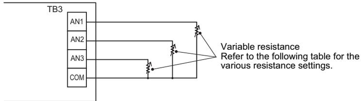
Do not apply voltage or current to AN1, AN2, AN3, or COM.
