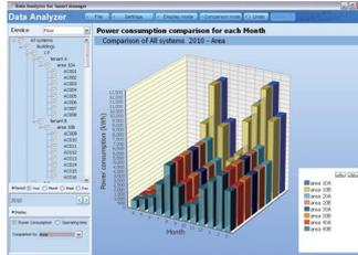
Power consumption of up to 4 floors displayed simultaneously in 3D graph.
