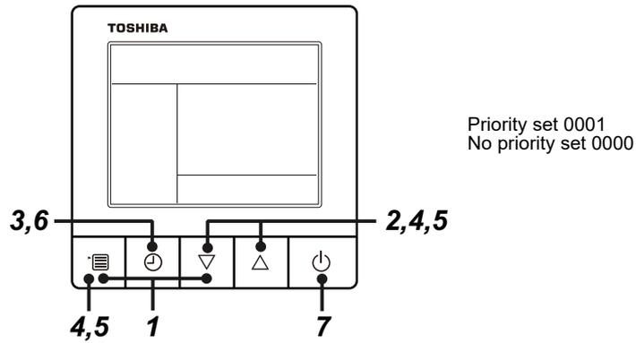
**1 Push and hold menu button and [ ∇ ] setting button simultaneously for 10 seconds or more.**
