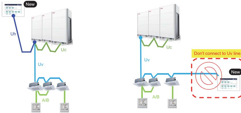
New Central remote controller can connect to TCC-LINK System. Then this device is restricted same as current model.
