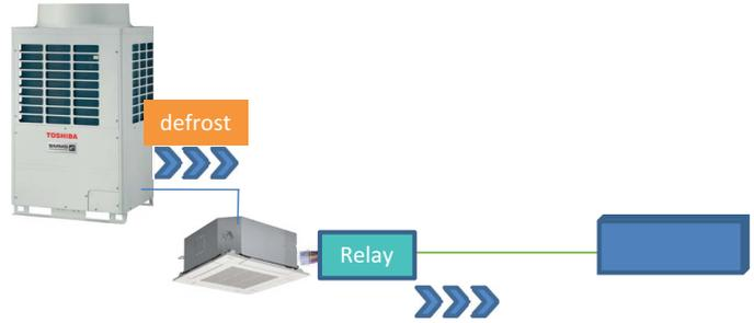
ON signal when indoor unit is "thermo-ON"
