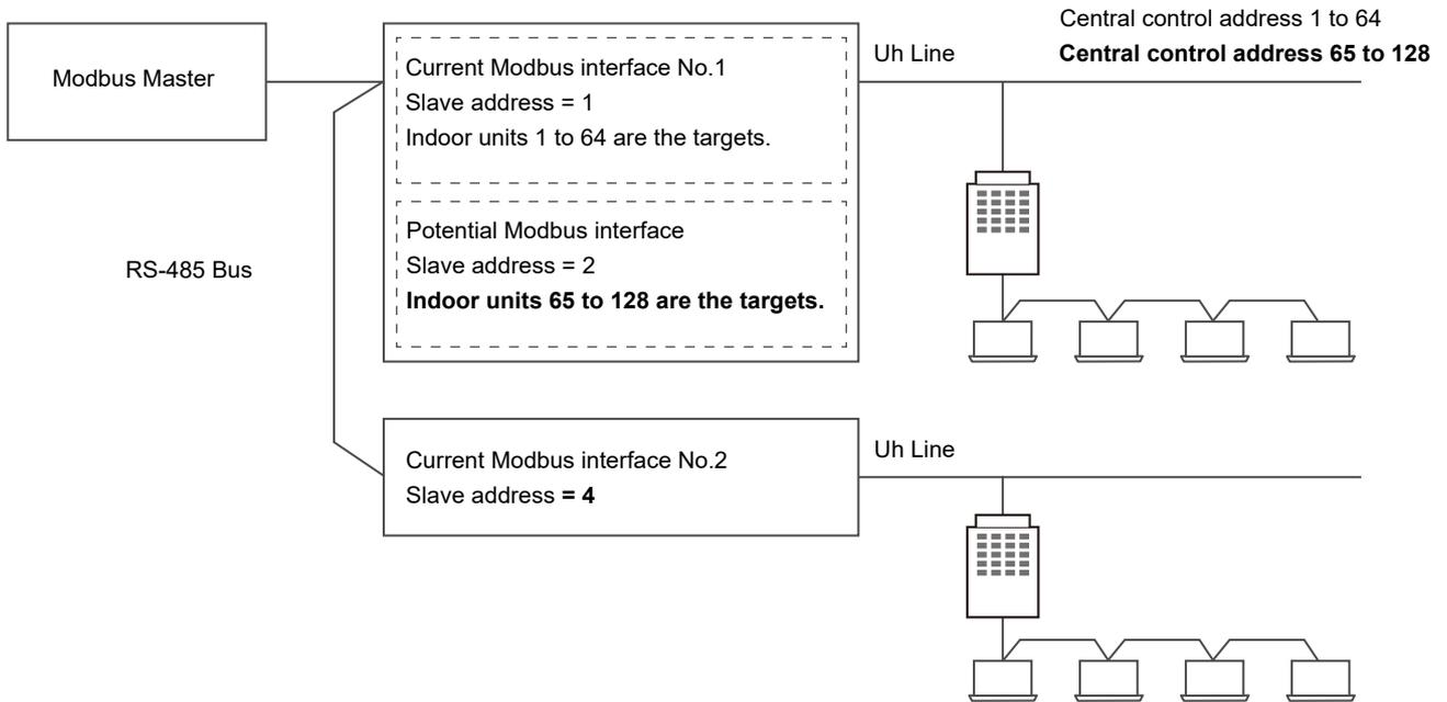
When two or more Modbus interfaces are connected to a single line RS-485 bus, set the slave addresses of the Modbus interface as indicated in the table below.
