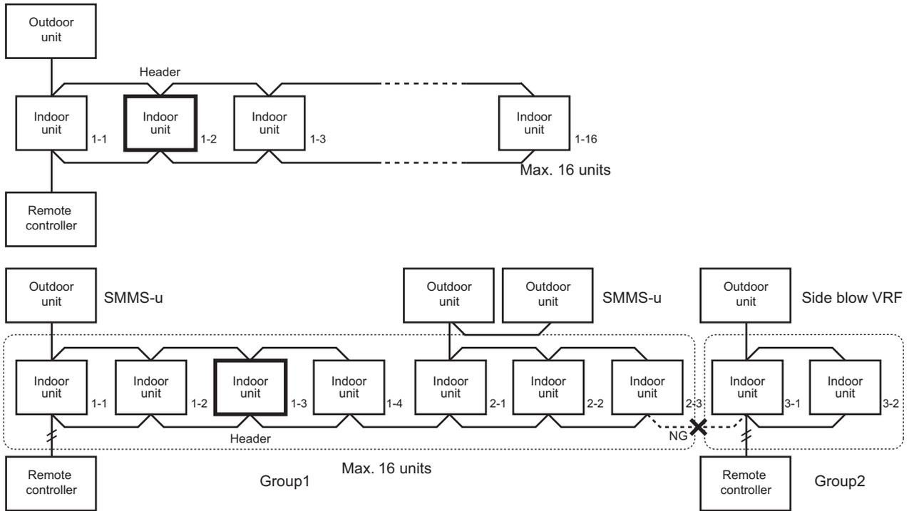
In case of DI/SDI, each Header indoor unit connected with outdoor unit controls room temperature according to setting on the remote controller. The Header indoor unit in the group is the representative of multiple indoor units and sends/receives signals to/from the remote controller and other indoor units in the group.
