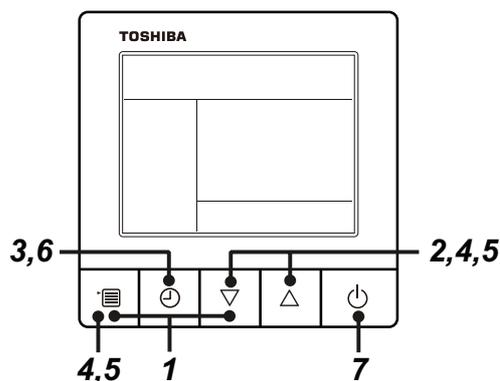
**1 Push and hold menu button and [ ∇ ] setting button simultaneously for 10 seconds or more.**
