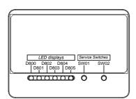
\* The LEDs and switches are locate at the Sub P.C.Board of the outdoor unit as shown in the figure on the left.
