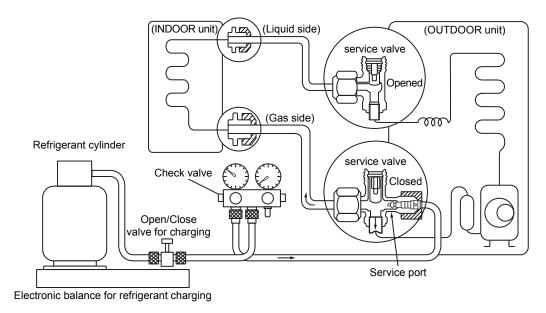
Fig. 6-4-1 Configuration of refrigerant charging
