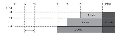
\* From 10 minutes to 15 minutes after a heating operation started, the minimum value of TE is stored in memory as TEO and the minimum temperature of TO as ToO.
