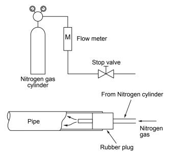
Fig. 6-5-1 Prevention of oxidation during brazing
