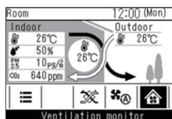
\*If you select the fan speed “Auto”, The fan speed is changed automatically in 7 stages according to the CO<sub>2</sub> concentration and PM2.5 concentration.
