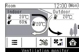
When is displayed on the detailed display, clean the filters.
