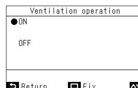
**1 In the "Ventilation" screen, push [ ▲ ] and [ ▼ ] to select "Ventilation operation", and then push [ Set/Fix]**
