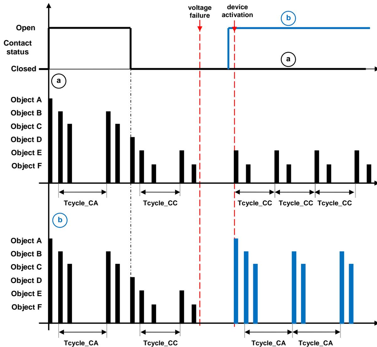
In the example above, objects A, B, C are sent on the contact opening edge and objects B and C are also sent cyclically. Objects D, E, F are sent on the contact closure edge and objects E and F are also sent cyclically. Chart "a" shows the condition in which the contact status when the device is activated following BUS voltage failure is the same as before that failure; vice versa, in chart "b" the contact status when the device is activated is different from that prior to the failure.
