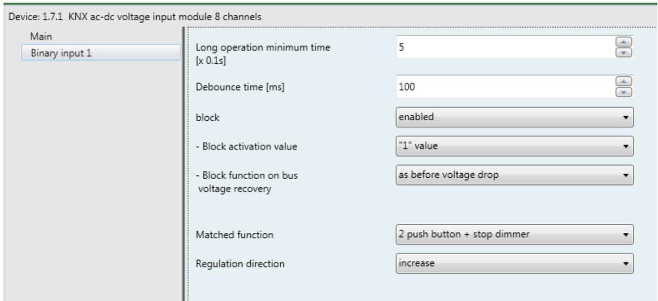
Fig. 4.6: "2 push button + stop dimmer" matched function menu
