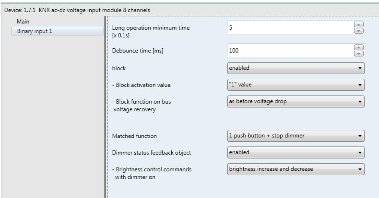
Fig. 4.3: "1 push button + stop dimmer" matched function menu
