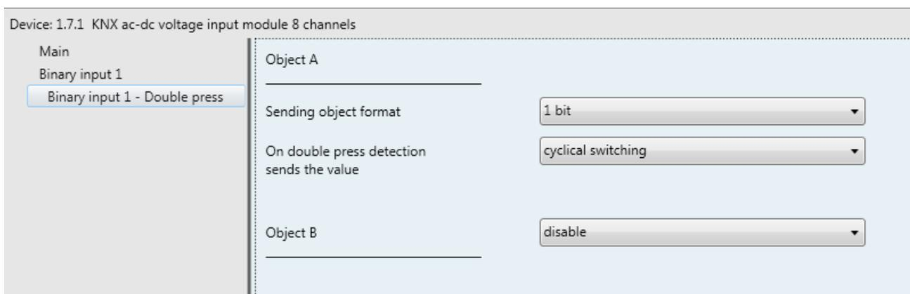
Fig. 4.16: “Binary input x – Double press” menu
