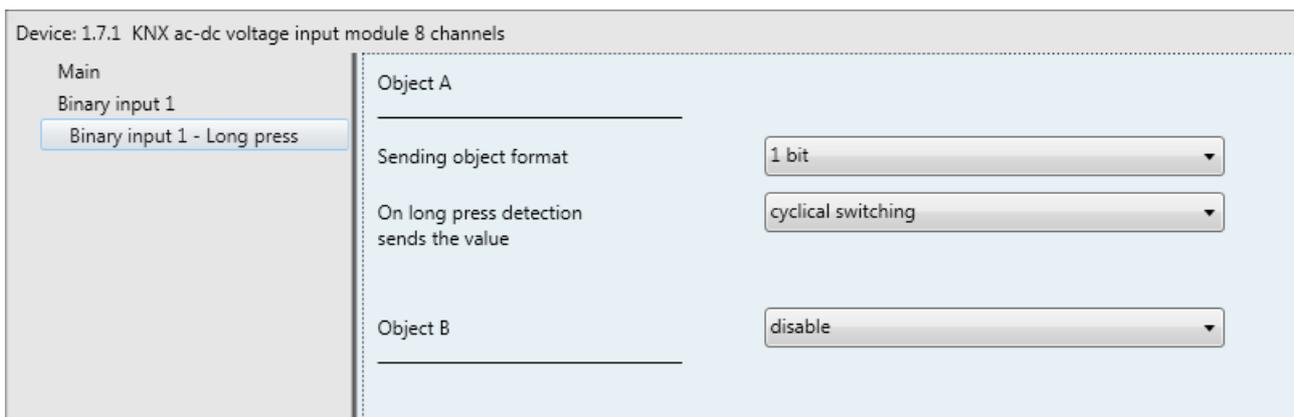
Fig. 4.19: “Binary input x – Long press” menu
