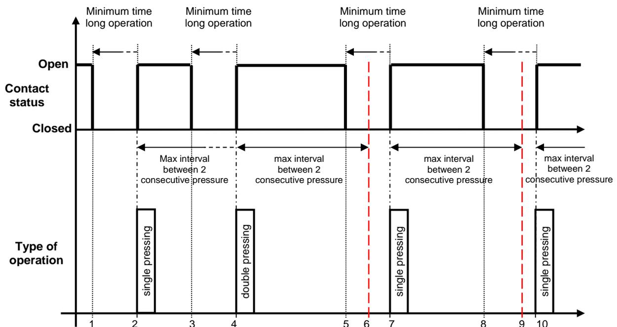
1. Once the closure of the contact has been detected, the contact closure time is calculated in order to distinguish a short press from a long one.
