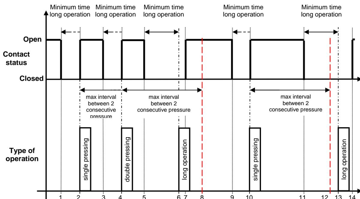
1. Once the closure of the contact has been detected, the contact closure time is calculated in order to distinguish a short press from a long one.
