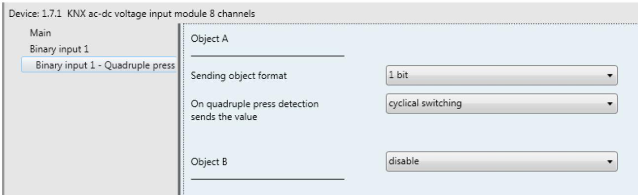
Fig. 4.18: “Binary input x – Quadruple press” menu
