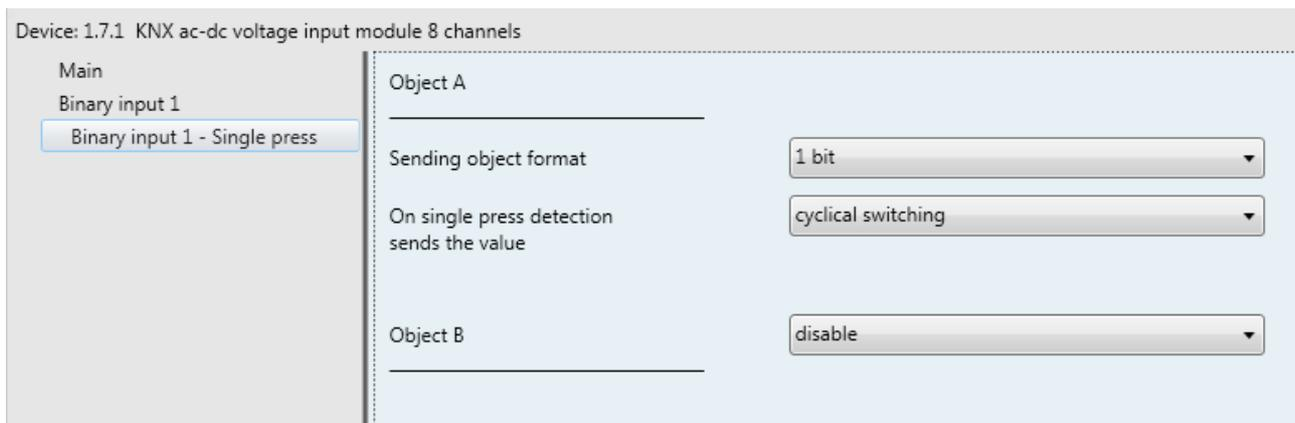
Fig. 4.15: “Binary input x – Single press” menu
