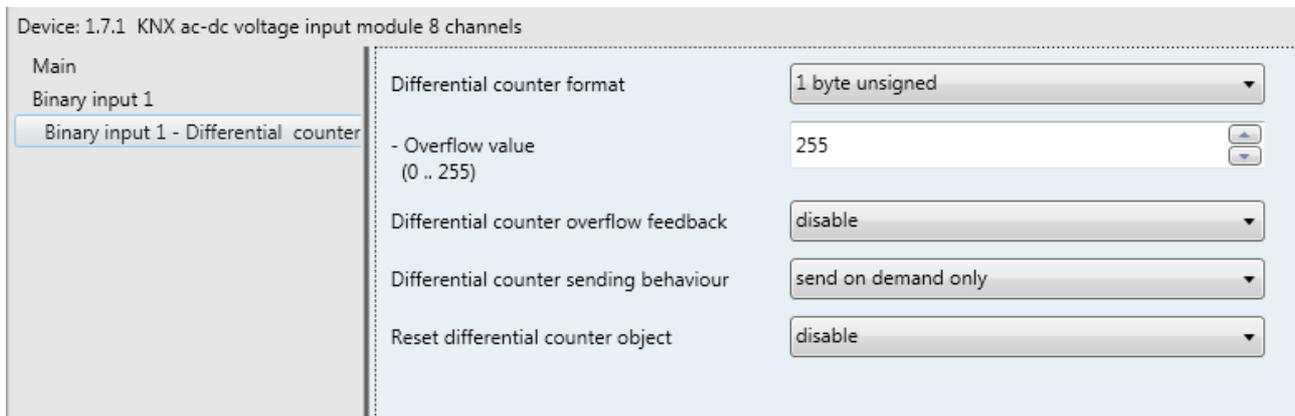
Fig. 4.13: “Binary input x – Differential counter” menu
