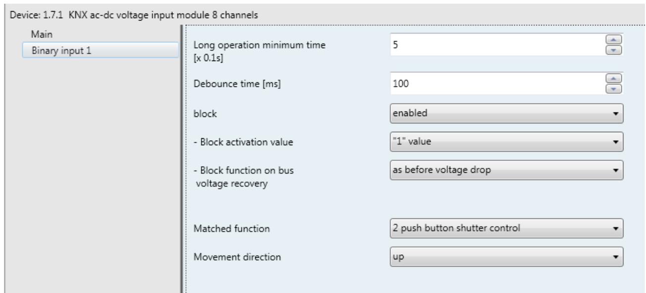
Fig. 4.8: "2 push button shutter control" matched function menu
