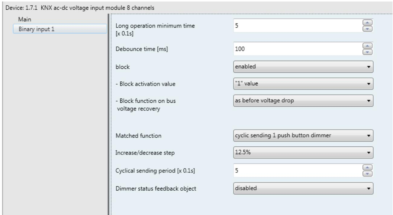
Fig. 4.4: "Cyclic sending 1 push button dimmer" matched function menu
