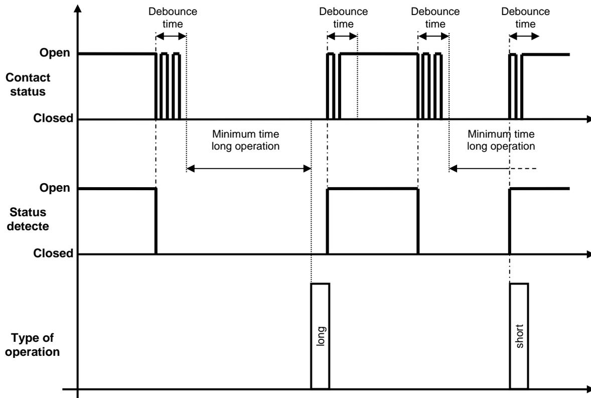
Starting from the top, the first chart shows a simulation of the time trend of the push-button status. The second chart shows the time trend of the push-button status detected by the device software that filters the contact disturbance (bounce) for a time equal to  $T_{\text{debounce}}$  starting from the moment when the first variation is detected.
