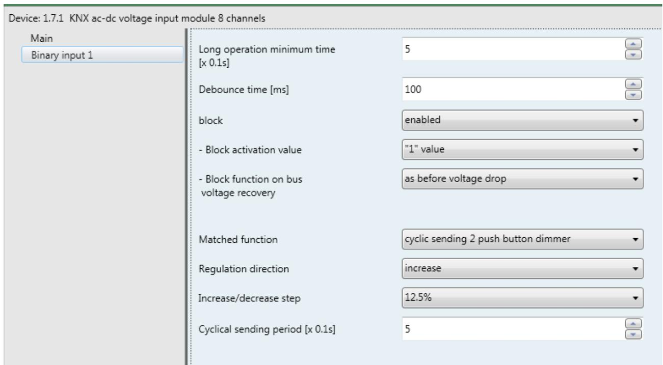
Fig. 4.7: "Cyclic sending 2 push button dimmer" matched function menu
