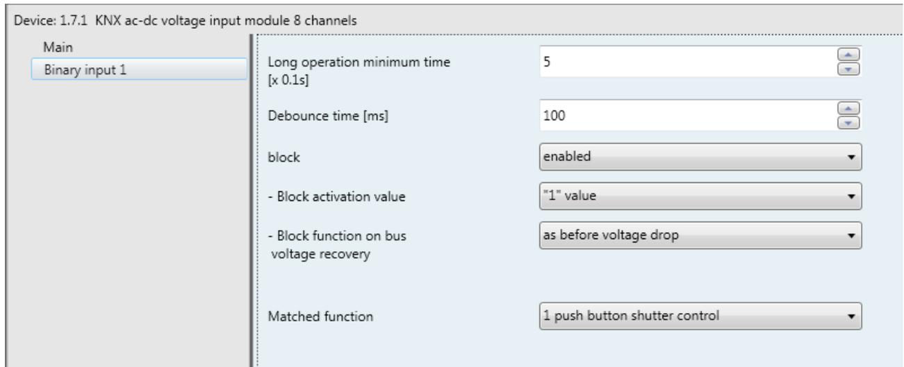
Fig. 4.5: "1 push button shutter control" matched function menu
