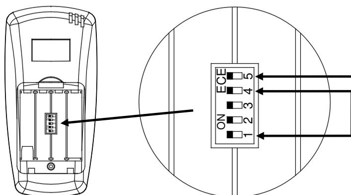
OFF-5-DIMMER: Seulement pour les ampoules à incandescence, halogènes, ...
