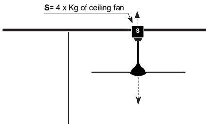
**i** **⚡** The support must support at least 4 times the weight of the fan.
