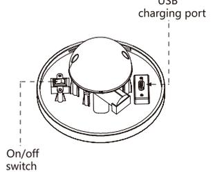
Turn on to activate the lamp. The lamp only can be charged when light off.
