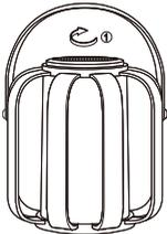
Twist clockwise to loosen
