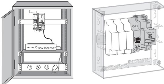
Tydom Pro must be installed on a DIN rail, either within a consumer unit, or in a VDI cabinet. The equipment must be installed by a suitably qualified person. Tydom Pro must be protected by a 2A circuit breaker, which will also serve as a power switch. Avoid proximity with power controls (of the type used for domestic hot water contactors)
