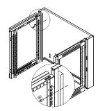
Install side frames to the grooves of back frame by 4pcs of M6\*12 screws (6pcs if more than 18U) as shown by the arrow in the picture, note 19" mounting rails are in the front side.
