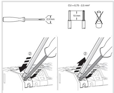
Fig 3: installation/deinstallation with plug-in terminals
