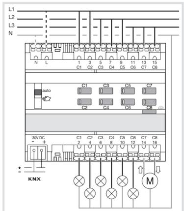
Fig 2: Device connection
