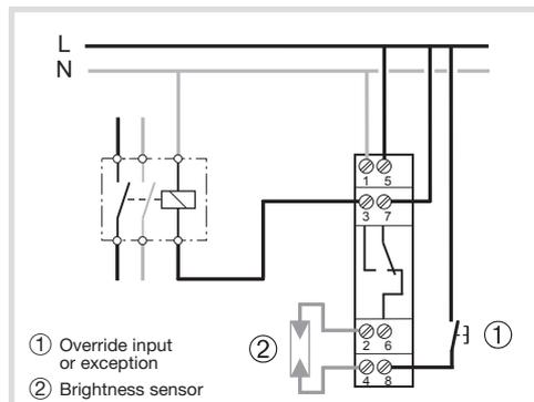
Figure 2: EGN100 connection diagram (1 output)
