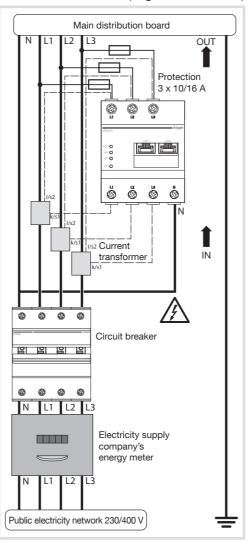
Use HAGER brand current transformers with a secondary current of 1A or 5A.
