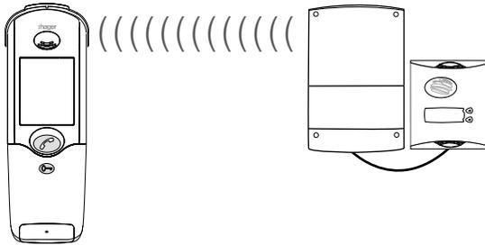
The Light button on the handset controls the lighting connected to the relay output receiver. The handset is considered as the transmitter while the output receiver acts as the receiver.
