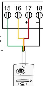
**TIP:** if the cable between the outdoor caller unit and the controller has to be lengthened, cut it at a distance of 1 m and then extend the red and black wires according to the rules below:
