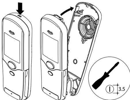
3. Replace the flat MTU01X battery with a new one.
