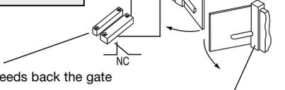
The position contact feeds back the gate status to the screen:
