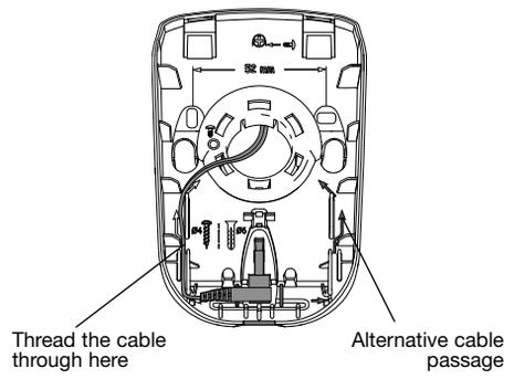
11. Thread the power cable into one of the guides at the back of the base.
