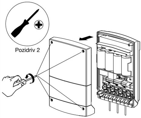
2. Replace the 4 flat LR20 batteries with new ones.
