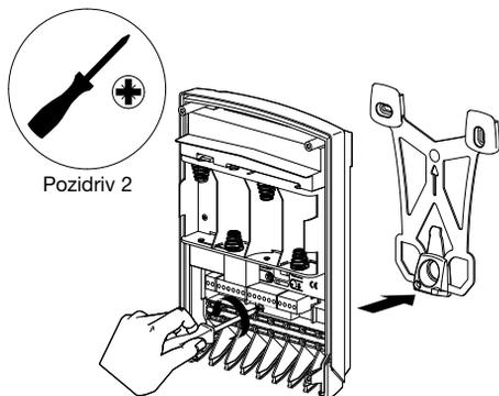
2. Following the installation rules below, mark 3 fixing points and drill a hole in the pillar using a  $\varnothing$  6 mm drill bit.
