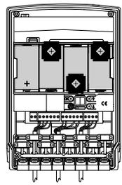
3. When the controller is powered, the radio link LED lights up red for 2 sec, the outdoor caller unit lights up and also beeps for 2 sec. If this is not the case, check the batteries have been correctly inserted.
