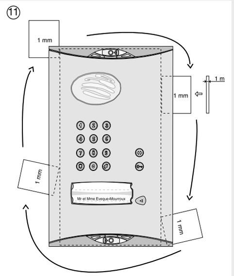
**IMPORTANT:** when the armoured cover is positioned on the unit, there should be a 1 mm clearance (use the shim for this purpose) between the pillar and armoured cover.
