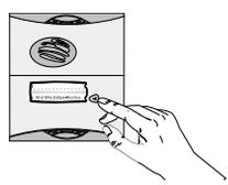
**IMPORTANT:** when using a translucent MHF01X or MHF02X outdoor caller unit and 1-button armoured cover, only the bottom key (KEY 1) can be accessed once the armoured cover has been placed on the unit.
