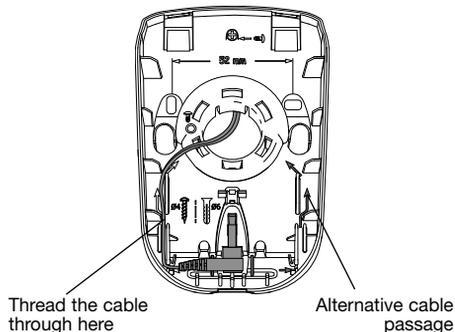
6. Thread the power cable into one of the guides at the back of the base.
