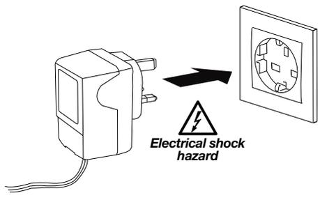
**IMPORTANT:** the mains socket must remain accessible so that the power pack can be easily disconnected.
