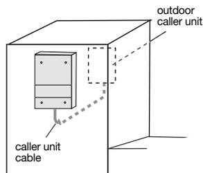
Do not place the products near metal surfaces (screens, fences, gates, etc.) or sources of electromagnetic disturbance:
