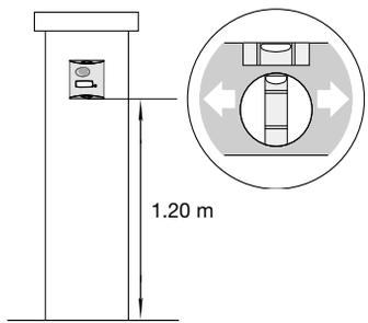
2. Mark and drill the outdoor caller unit holes with a Ø 6 mm drill bit. Also mark the place where the cable feed hole has to be drilled (Ø 8 mm min. recommended).
