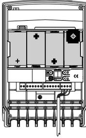
**IMPORTANT:** push the batteries into their slot making sure that the + pole of each one is in contact with the metal part.
