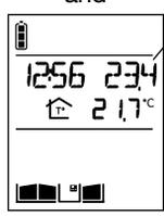
Display of time, indoor and outdoor temperature, gate, side gate and latch status (if position contacts connected).
