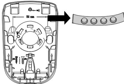
3. Rotate the back of the base until it is in "table" position.
