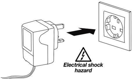
**IMPORTANT:** the mains socket must remain accessible so that the power pack can be easily disconnected.
