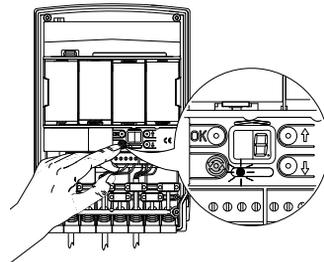
4. Press and hold
