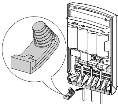
4. Use the cable clamp and screws provided to lock the cables in place.
