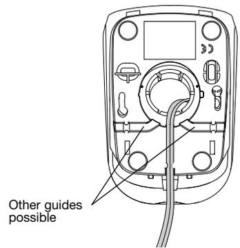
12. Fix the base to the wall using appropriate washers and screws.
