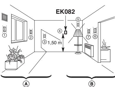
Install the probe at 1,50 m from the floor, ④ on the internal wall, avoiding external influences: (① extraction fan, ② external wall, ③ sunlight) and internal influences: (⑤ lighting device, ⑥ chimney, electrical ⑦ heater)
