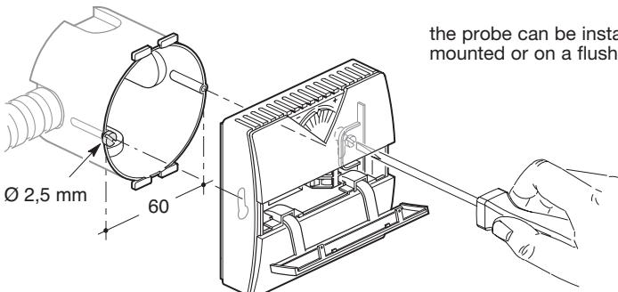
the probe can be installed either surface mounted or on a flush box
