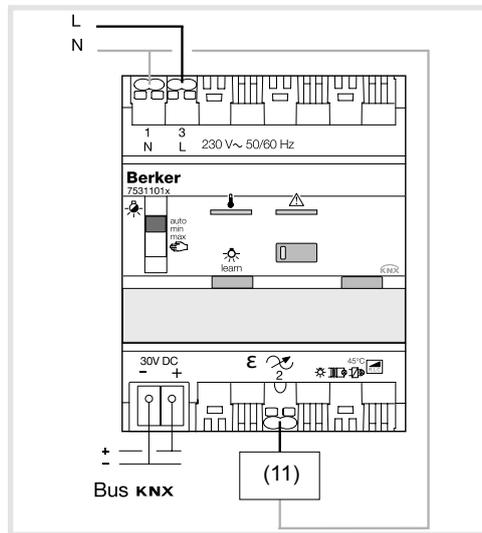
Fig 3: Device connection
