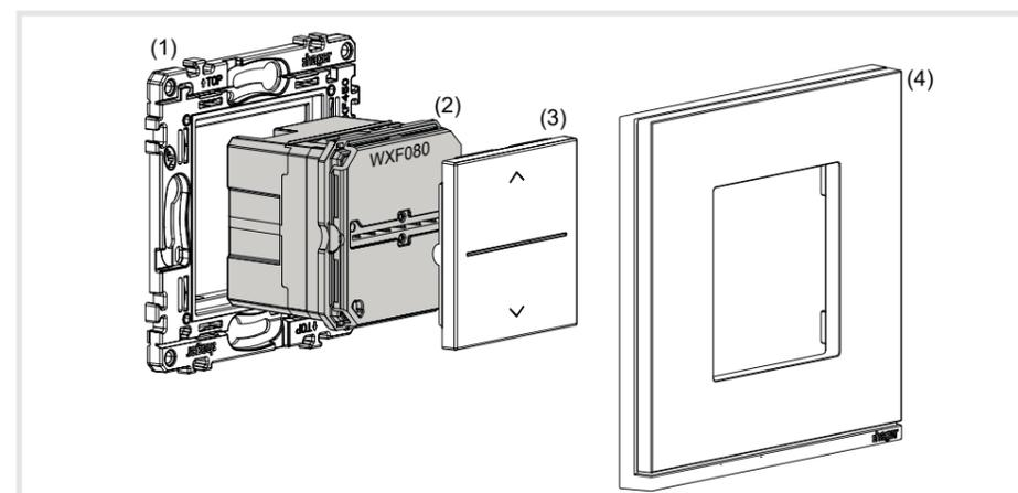
Figure 1: Design and layout of the device
