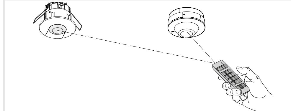
**(EN)** The remote control allows the user to set or modify settings on the presence detectors (see above). When the potentiometer is on "auto test". It allows single and multiple settings. The SET key is used to send the IR messages to the occupancy sensors. Multiple settings can be stored in Memo 1 and Memo 2 and recalled to set several devices.
