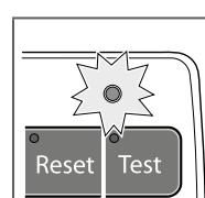
The acknowledgment LED blinks during the sending of the IR message.
