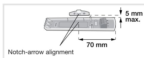
**!** Side alignment and height adjustment are required for correct operation of the detector.
