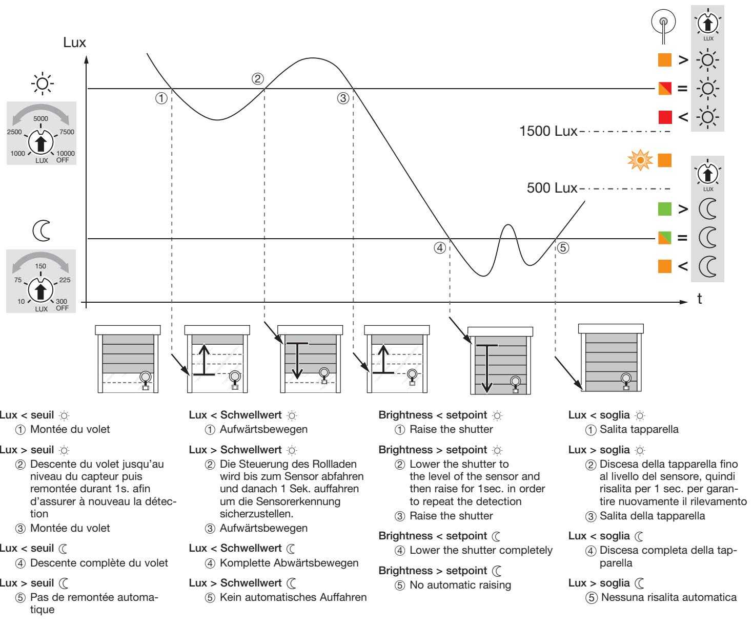
**E Configuration quicklink volet/Rollladen quicklink-Konfiguration/Shutter quicklink configuration/Configurazione quicklink tapparella**
