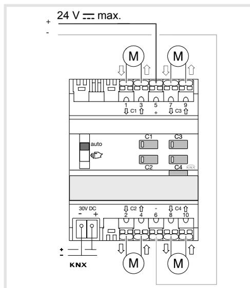
Fig 2: device connection
