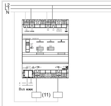
Figure 4: Device connection multi-phase
