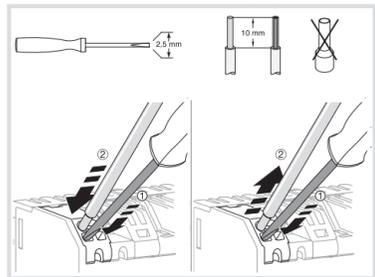
Fig 2: Installation/removal with plug-in terminals
