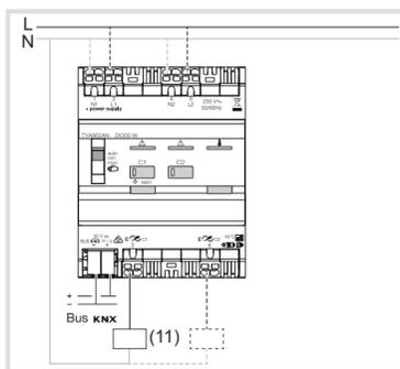
Figure 3 : Device connection 1-phase
